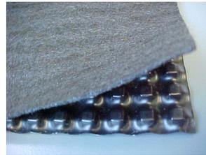
**EARTH DRAIN II** is .25 inch thick with 1/2 inch center-to-center peg spacing. Ideal for projects requiring lower flow rates and a higher compressive strength.
