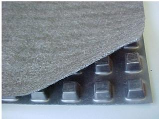
**EARTH DRAIN** is .42 inch thick with 1 inch center-to-center peg spacing. Ideal for projects requiring high flow rates with moderate compressive strength.
