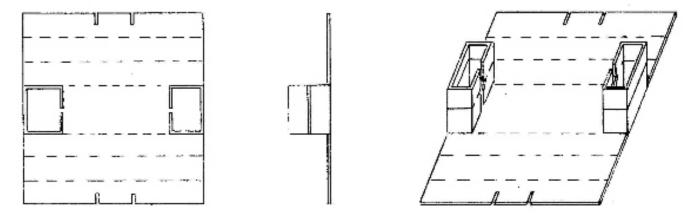
Take box shaped ends from step 2 and fold up 90 degrees until inside of box is flush with cover sheet, as shown.
