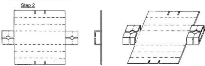
Form both end panel into box shape as shown:
