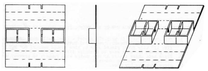
Fold top of box shaped ends 180 degrees toward center of form until flush with cover sheet, as shown.
